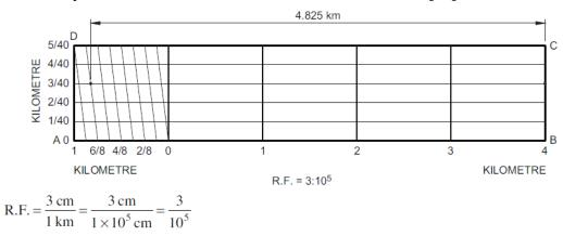
Since scale has to show a distance of 4.825 km, the maximum length should be at least 5 km. Length of scale,  $L_s = \text{R.F.} \times \text{Maximum length} = \frac{3}{10^5} \times 5 \times 10^5 \text{ cm} = 15 \text{ cm}$ The breakup of 4.825 km is  $4 \text{ km} + 6 \times \frac{1}{8} \text{ km} + 3 \times \frac{1}{40} \text{ km}$ .
