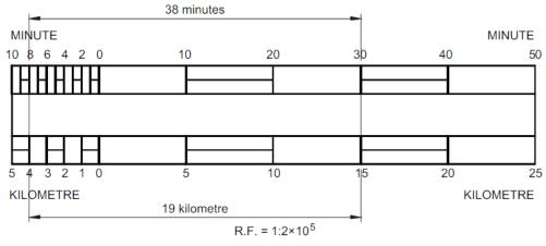
The distance covered in 1 hour = 150/5 = 30 km. Length of scales,  $L_s = R.F. \times Maximum$  length
