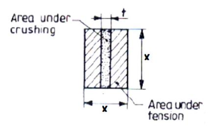
3. Compression / Crushing Failure of rod and Cotter
