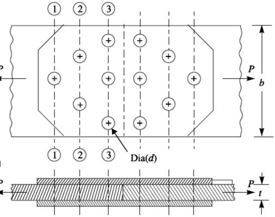
Riveted Joint for Structural Use–Joints of Uniform Strength (Lozenge Joint)
