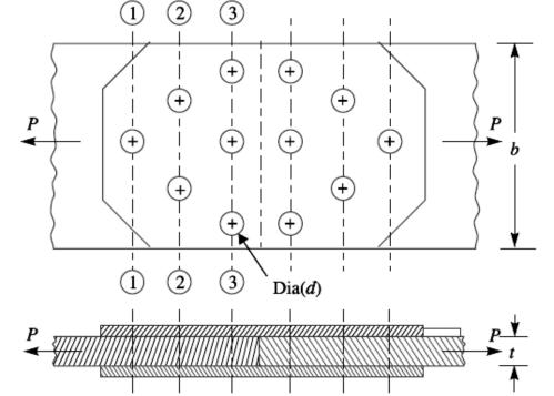
In diamond riveting, the number of rivets increases as we proceed from the outermost row to the innermost row.
